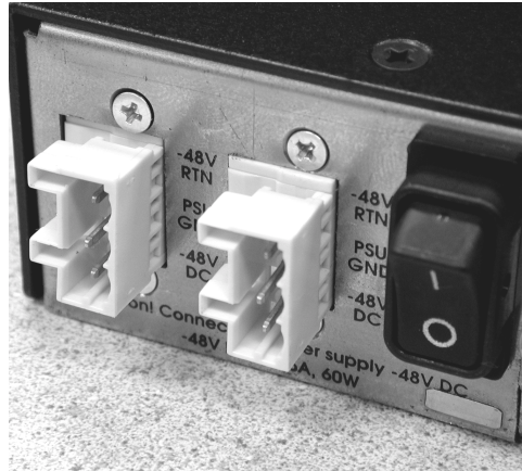
DC power inputs
